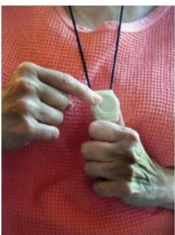
**Landline System:** When the call button is pressed, an alarm signal is sent to the control panel in your home, which automatically calls our monitoring center. The dispatcher will follow your predetermined instructions and
